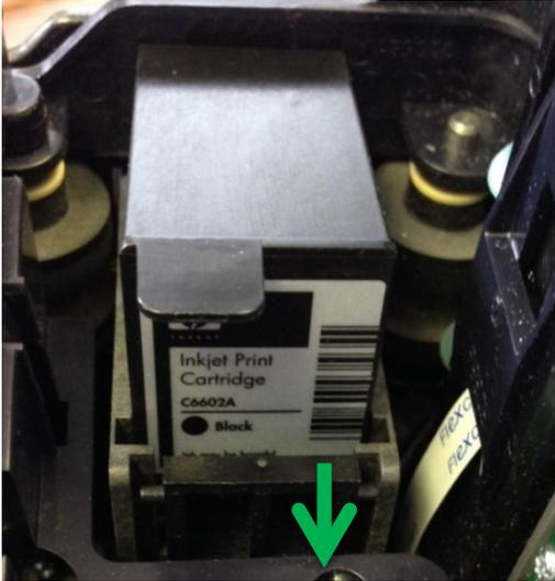
3. Pull the inkjet cartridge out of the scanner.
