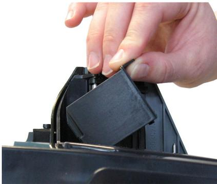
5. Push the cartridge down into the holder until the cartridge snaps into place. Once installed, the inkjet cartridge sits on a slight angle with the back of the cartridge lower than the front.
