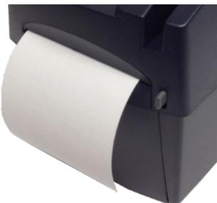
Make sure the cover is completely closed. If you push the cover from the sides, the cover might not close completely. When closed correctly, both sides of the printer cover are flush with the scanner.
